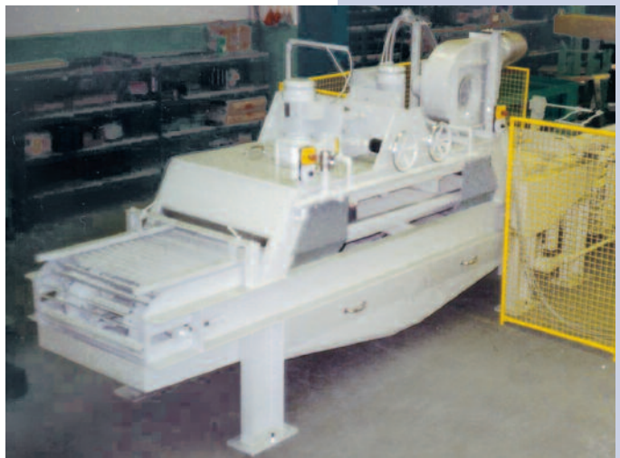
RWM washing lines for small-grained and coarse-grained washed-out concrete
